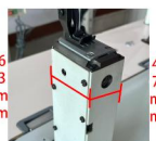
Post bed size: 63mm, 47mm 柱子尺寸: 63mm, 47mm
