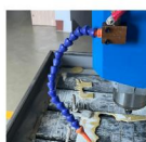
Circulation water pipe 循环出水管
