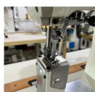
Presser foot picture 压脚图片
