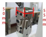
Post bed size: 50mm, 55mm 嘴巴尺寸: 50mm, 55mm
